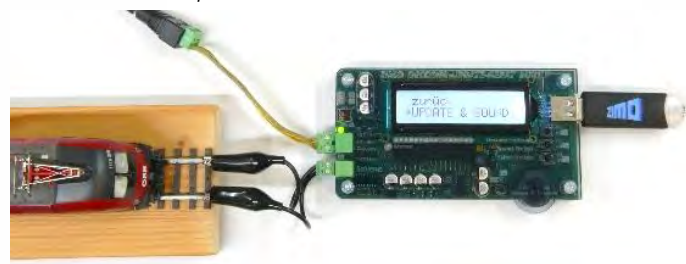
For the self-update, only the power supply (at terminal "Power" of the MXULFA) must be connected, and a USB stick with the correct files for the update must be inserted.
