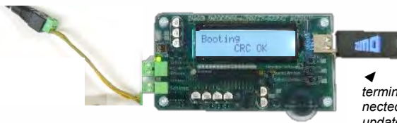
Typical arrangement for software update and/or sound loading via "rail": Decoder installed in locomotive, locomotive on "update track", power supply from power supply unit via terminal "Power", USB stick with the correct files for update and/or sound loading inserted.
